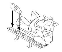
Figure 54 - Installing Log No. 5
